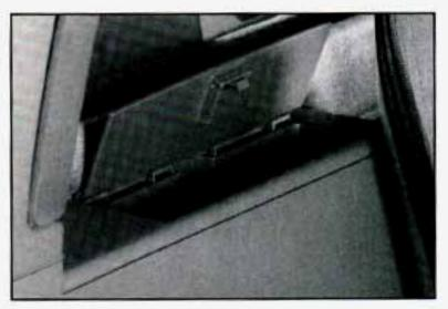
If you have a rear storage compartment, pull up on the handle to open or remove the cover. To replace the cover, fit the notches on the cover into the storage compartment slots and push down.
